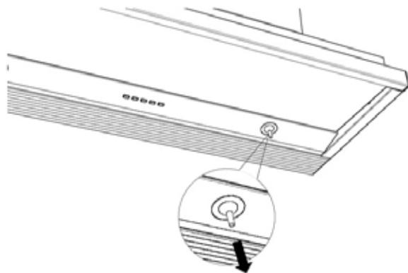
A suction cup for removing the lamps has been delivered with the hood. Place the suction cup onto the halogen spot and draw it towards you. The lamp will now come out. You can also install the new lamp using the suction cup.
