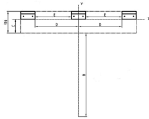
See the table for mounting the attachment brackets. Note the appropriate type number of the extractor hood!
